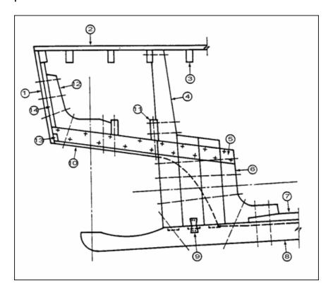
**6.** In the following sketch of a typical stem assembly of a timber vessel, name the numbered parts.
