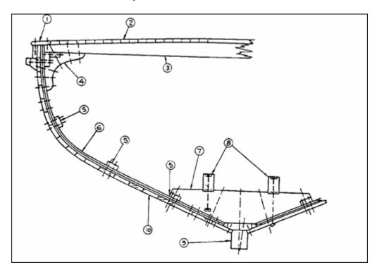
**5.** In the following sketch of a typical deadwood aft, name the numbered parts.
